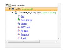
If a connection cannot be made between Leapfrog Geo and ioGAS, it could be that the **Timeout** setting in ioGAS is too low. To change this, navigate to the folder C:\Users\....\AppData\Roaming\ioGAS\userConfig. Open the file link.ini in a text editor and set the **Timeout** parameter to a higher value. The **Timeout** is in milliseconds.
