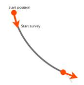
The algorithm matches the survey at the starting and end positions exactly and the curvature is constant between these two measurements. At the survey points, the direction remains continuous and, therefore, there are no unrealistic sharp changes in direction.
