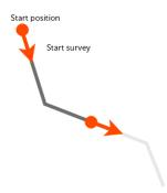
It is an improvement on the raw tangent algorithm but still suffers from an unrealistic discontinuity in the drillhole path. It is, however, a better approximation of the overall drillhole path and is reasonably accurate when the spacing between measurements is small.
